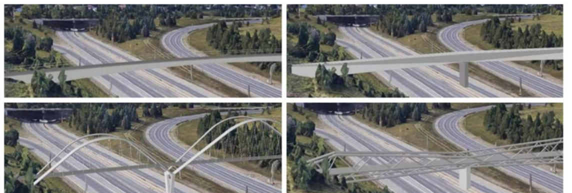
The Expansion Program includes a pedestrian and cyclist bridge over Whitemud Drive that will connect the neighbourhoods of Brookside and Brookview. Options include truss, girder and arch designs.
