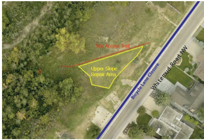
This view shows the area where access trail restoration and slope repair work will be carried out at the Whitemud Road landslide site.
